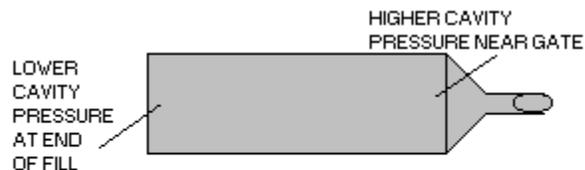
End gating long thin parts minimizes warpage by providing a gradual pressure drop across the cavity.
